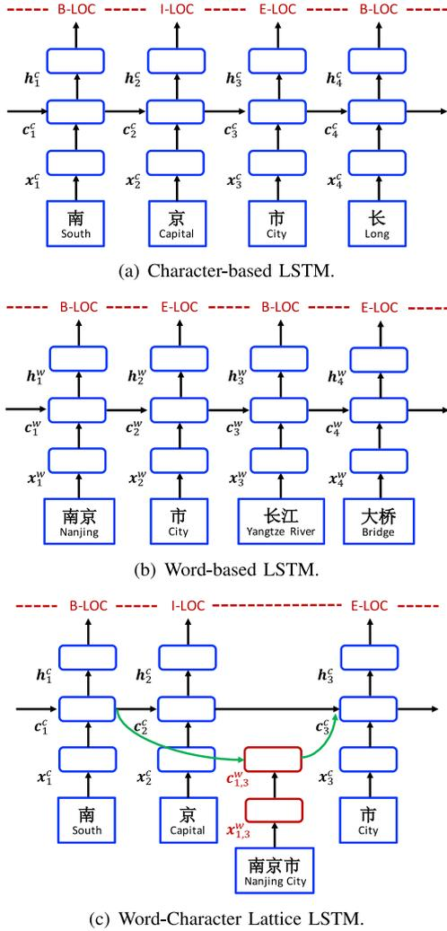
Fig. 3. Word/character LSTM and word-character lattice LSTM Models.
