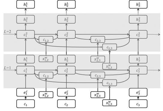
Fig. 4. The structure of multi-layer stacked lattice LSTM.
